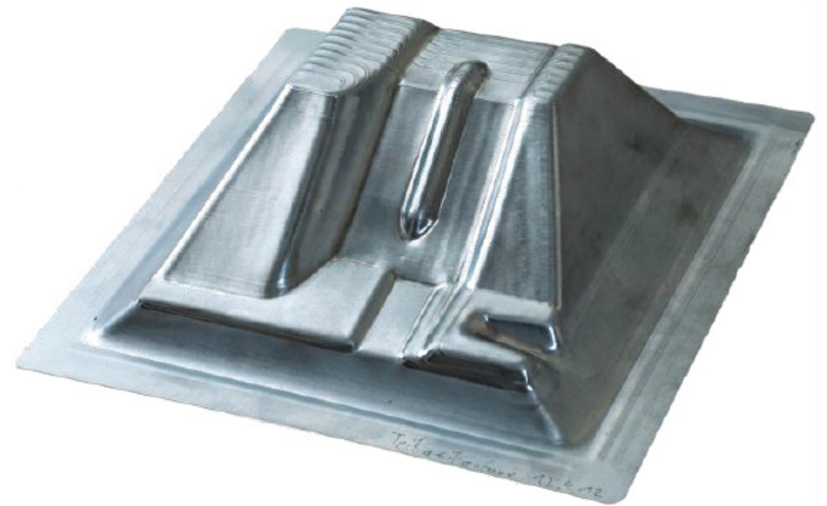
Part formed with Roboforming with Local Support
