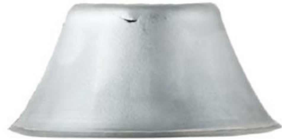
Point of Failure with Peripheral Support
