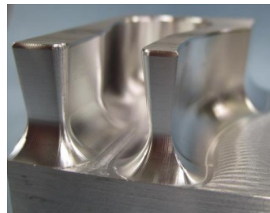
Undercuts made with a 5-axis Mill Image credit: onecnc.net/
