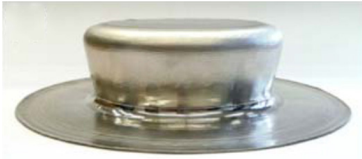
Cylinder with Undercut (97°) Image credit: (Meier et al., DPF, 328)
