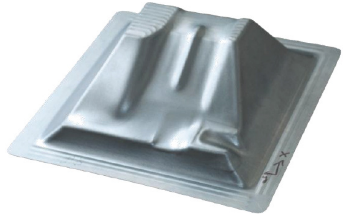
Part formed with Single Point Incremental Forming
