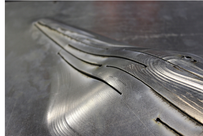
Incrementally Form -> 3D Plasma Cut -> Incrementally Form
