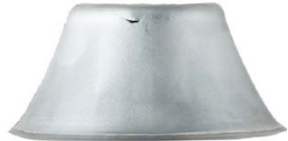
Point of Failure with Peripheral Support
