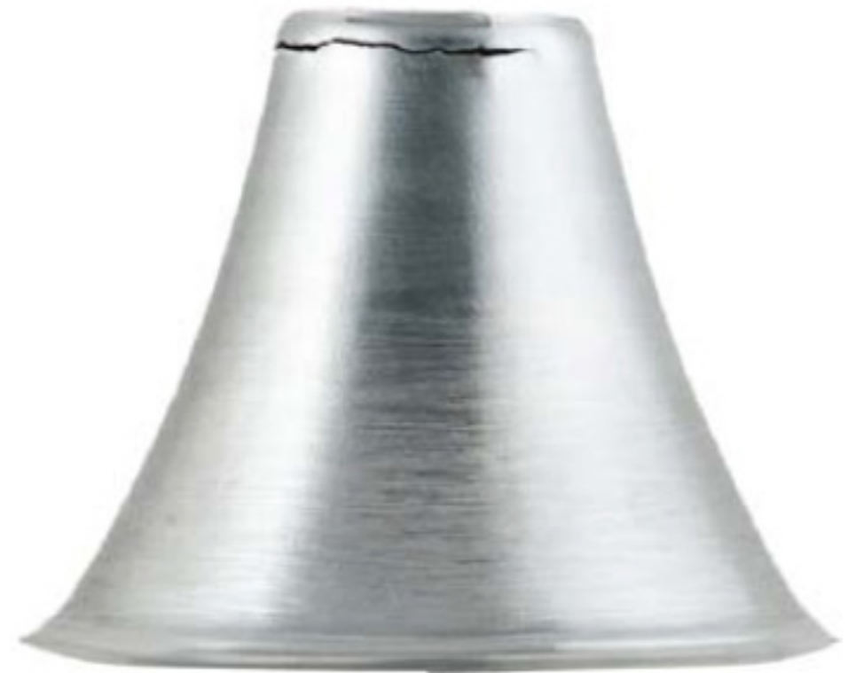
Point of Failure with Local Support
